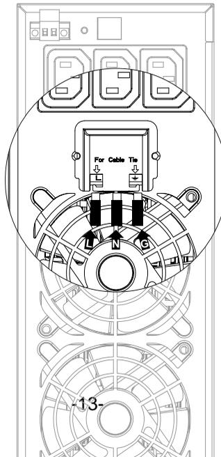
■ **Figure 5.1 Output Connection diagram of 3KL T IEC model**
